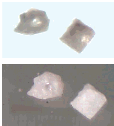
Figure 2. TGA samples (top, transmitted light; bottom, reflected light; scale same as that as for Figure 1c) showing ex-solution glass globules on ALPO orthoclase pseudomorphs of PSU-2.
